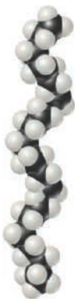
▲ Figure 12.39 A segment of a polyethylene chain. This segment consists of 28 carbon atoms. In commercial polyethylenes, the chain lengths range from about 10^3 to 10^5 \text{CH}_2 units.
