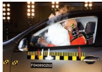
▲ Figure 3.7 Decomposition of sodium azide, \text{NaN}_3(s) , produces \text{N}_2(g) that inflates air bags in automobiles.
