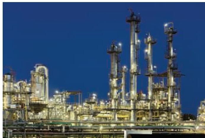
▲ Figure 13.19 The volatile components of organic mixtures can be separated on an industrial scale in these distillation towers.
