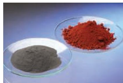
▲ Figure 2.22 Different ions of the same element have different properties. Both substances shown are compounds of iron. The grey substance on the left is \text{Fe}_3\text{O}_4 , which contains \text{Fe}^{2+} and \text{Fe}^{3+} ions. The red substance on the right is \text{Fe}_2\text{O}_3 , which contains \text{Fe}^{3+} ions.
