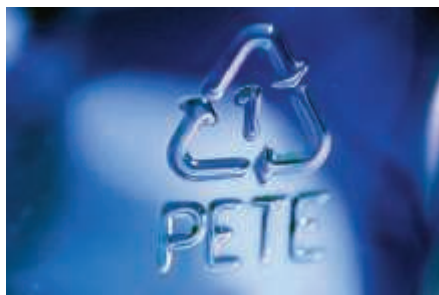
▲ Figure 12.34 Recycling symbols. Most plastic containers manufactured today carry a recycling symbol indicating the type of polymer used to make the container and the polymer’s suitability for recycling.
