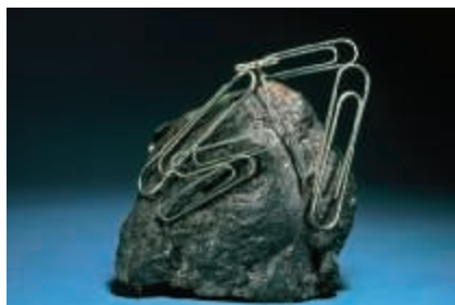
▲ Figure 23.7 A permanent magnet. Permanent magnets are made from ferromagnetic and ferrimagnetic materials.
