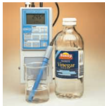
▲ Figure 16.7 A digital pH meter. The electrodes immersed in a solution produce a voltage that depends on the pH of the solution.
