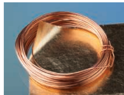
▲ Figure 12.10 Malleability and ductility. Gold leaf demonstrates the characteristic malleability of metals, and copper wire demonstrates their ductility.
