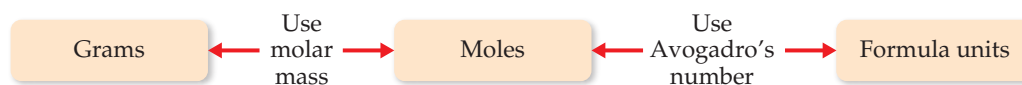
▲ Figure 3.12 Procedure for interconverting mass and number of formula units. The number of moles of the substance is central to the calculation. Thus, the mole concept can be thought of as the bridge between the mass of a sample and the number of formula units contained in the sample.
