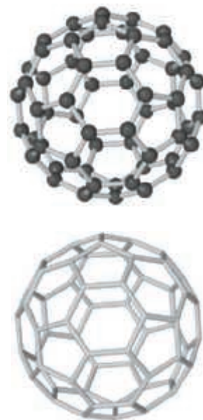
▲ Figure 12.49 Buckminsterfullerene, C_{60} . The molecule has a highly symmetric structure in which the 60 carbon atoms sit at the vertices of a truncated icosahedron. The bottom view shows only the bonds between carbon atoms.
