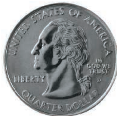
▲ Figure 2.15 The US quarter dollar is made from an alloy that is 91.67% Cu and 8.33% Ni.
