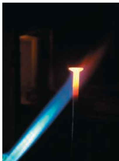
▲ Figure 6.5 Color and temperature. The color and intensity of the light emitted by a hot object, such as this nail, depend on the temperature of the object.
