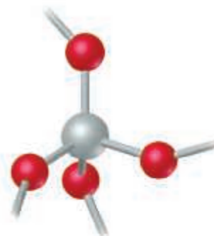
Fragment of extended \text{SiO}_2 lattice; Si forms only single bonds
