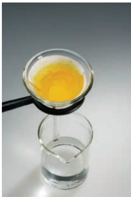
▲ Figure 1.12 Separation by filtration. A mixture of a solid and a liquid is poured through filter paper. The liquid passes through the paper while the solid remains on the paper.
