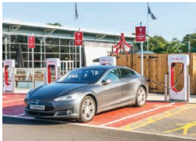
▲ Figure 20.22 Electric car. This Tesla electric automobile can go about 200 miles after 30 minutes of charging at this station.
