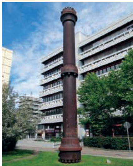
▲ Figure 15.5 A high-pressure steel reactor used in the Haber process is on display at Karlsruhe Institute of Technology in Germany where the Haber process was developed.
