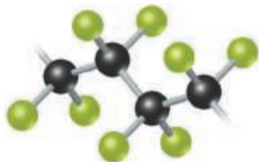
▲ Figure 22.9 Structure of Teflon®, a fluorocarbon polymer.
