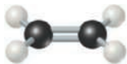
▲ Figure 9.21 Trigonal-planar molecular geometry of ethylene. The double bond is made up of one C—C \sigma bond and one C—C \pi bond.
